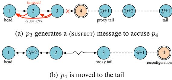
**Fig. 3.** Example (1). A faulty replica is denoted by a double circle. After the timer expires, replica  $p_3$  issues a  $\langle \text{SUSPECT} \rangle$  message to accuse  $p_4$  (which is faulty). The head moves  $p_3$  to the proxy tail position and the faulty replica  $p_4$  to the end of the chain.
