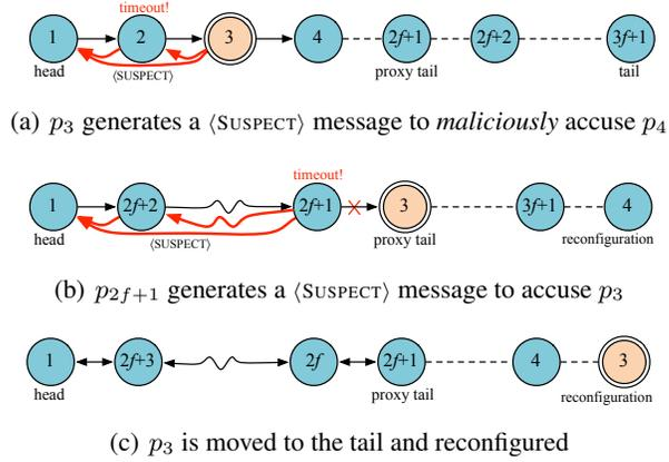
**Fig. 4.** Example (2). Replica  $p_3$  maliciously sends a  $\langle \text{SUSPECT} \rangle$  message to accuse  $p_4$ . The head moves  $p_3$  to the proxy tail and  $p_4$  to the end of the chain. If  $p_3$  does not behave, it will be accused by its predecessor  $p_{2f+1}$  such that in another round of re-chaining  $p_3$  is moved to the end.
